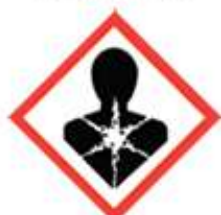
Serious health hazard
